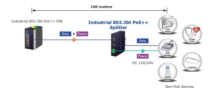
The POE-173S frees the network device deployment from restrictions of power outlet locations, thus eliminating the costs for additional AC wiring and reducing the installation time.
